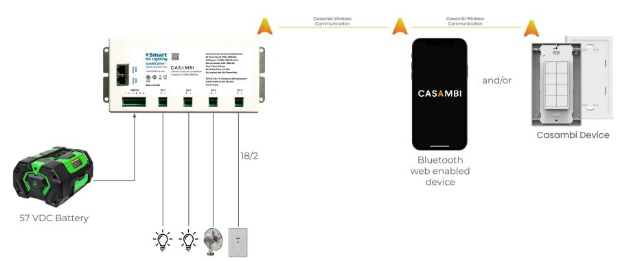
voltage of loads must be at least 3VDC less than the QDCD input power voltage
